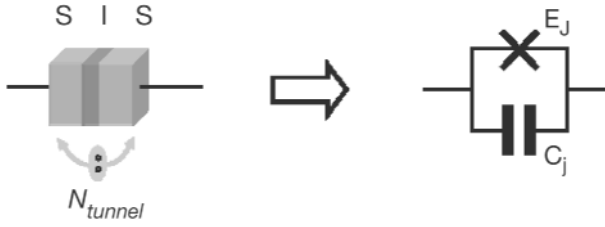
Fig. 9.1. A schematic representation of a Josephson junction and the equivalent circuit
